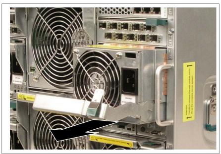
Figure 79: Removing the PSU
